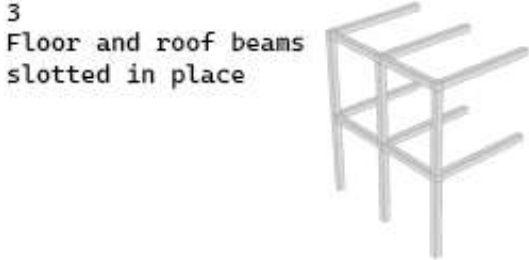
2 Horizontal beams slotted into place
